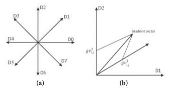
**Figure 18.** (a) Eight (D0–D7) chain code direction. (b) Breakdown of gradient vector.
